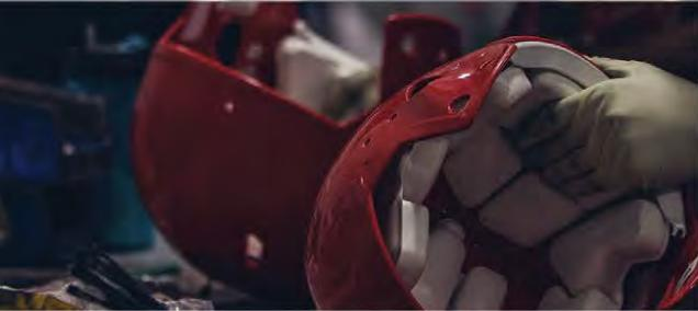
Helmets and shoulder pads are inspected for any wear and tear that might compromise protective performance.
